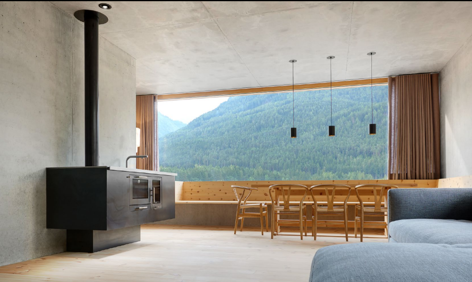
Kitchenstove tailor-made in natural steel and worktop in full stainless steel 8 mm
